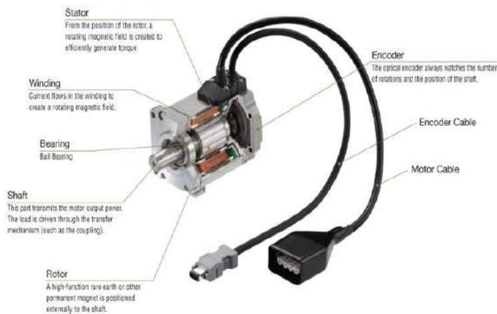
Fig.4: Parts of Servo motor
