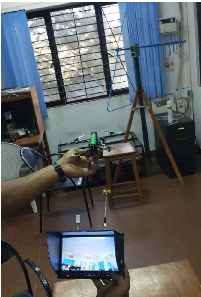
Fig 9: Assembly of Pagoda antenna for drone video reception.
