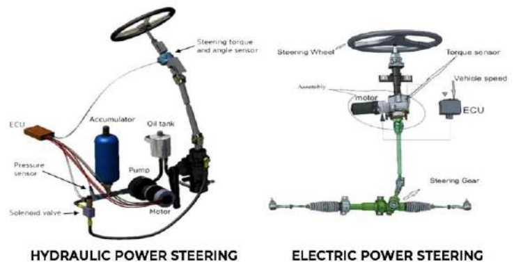
Figure 1. Electric vs hydraulic power steering
