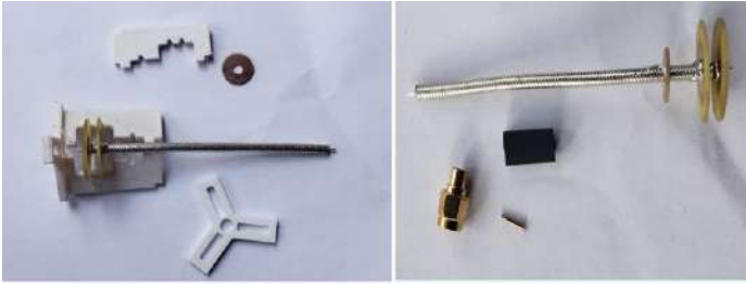
Fig. 8 Soldering using 3D printed Jig and SMA connector The assembled antenna was mounted on the FPV (First Person View) monitor as shown in Fig 9.
