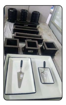
3 Nos. of Cubical moulds (150 mm x 150 mm x 150 mm, 3 Nos. of Cylindrical moulds (150 mm dia. and 300 mm height), 3 Nos. of Prism moulds (100 mm x 100 mm x 500 mm), Enamel Trays (3 Nos.) and 2 Nos. of trowels
