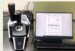
Fourier Transform Infra-Red (FTIR) Spectrometer Make: Agilent Model: Cary 630 FTIR Spectrometer
