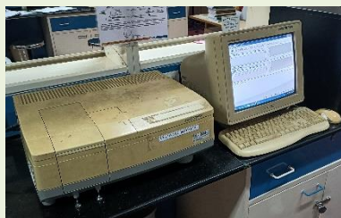
UV-VIS Spectrophotometer Make: Shimadzu Model: UV-1650PC
