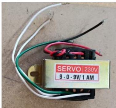
Fig. 14. Step down transformer.
