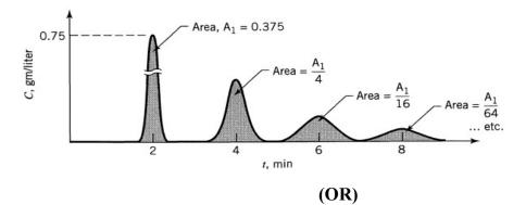
(b) A pulse input of tracer (M=13.5 μmol/s) into a vessel of volume 60 cm<sup>3</sup> gives (14) 3 4 the results as shown below. The results are found to be consistent by checking the material balance with the tracer curve. Construct E curve. Also calculate mean residence time.
